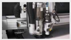
The EMH head allows to sequentially or separately use the cutting knife and the router. It is the best solution to combine the process of foam or rigid materials as well as to process a great number of other materials with a single tool. Two different types of routers are available: both turning at high-speed, with a power of 1 or 2.4 kW, air cooling system, variation of the speed rate during the processing and vacuum cleaning system with electric height regulation.
